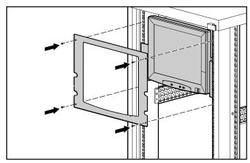
Figure 2-23. Attaching the faceplate
